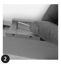
Position slider over plates (lock slider with grub screw/hex key).
